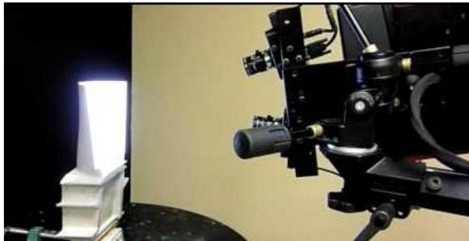
Fig. 16. White light scanner [14].
