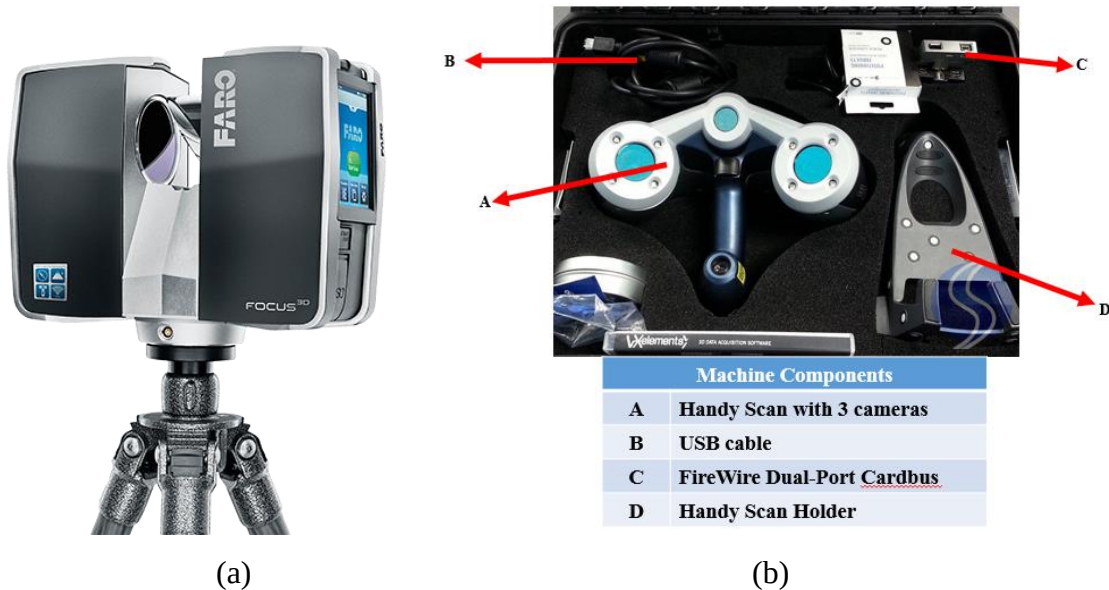
Fig. 18. (a) Tripod laser scanner [16], and the 3D scanner at RCAM.
